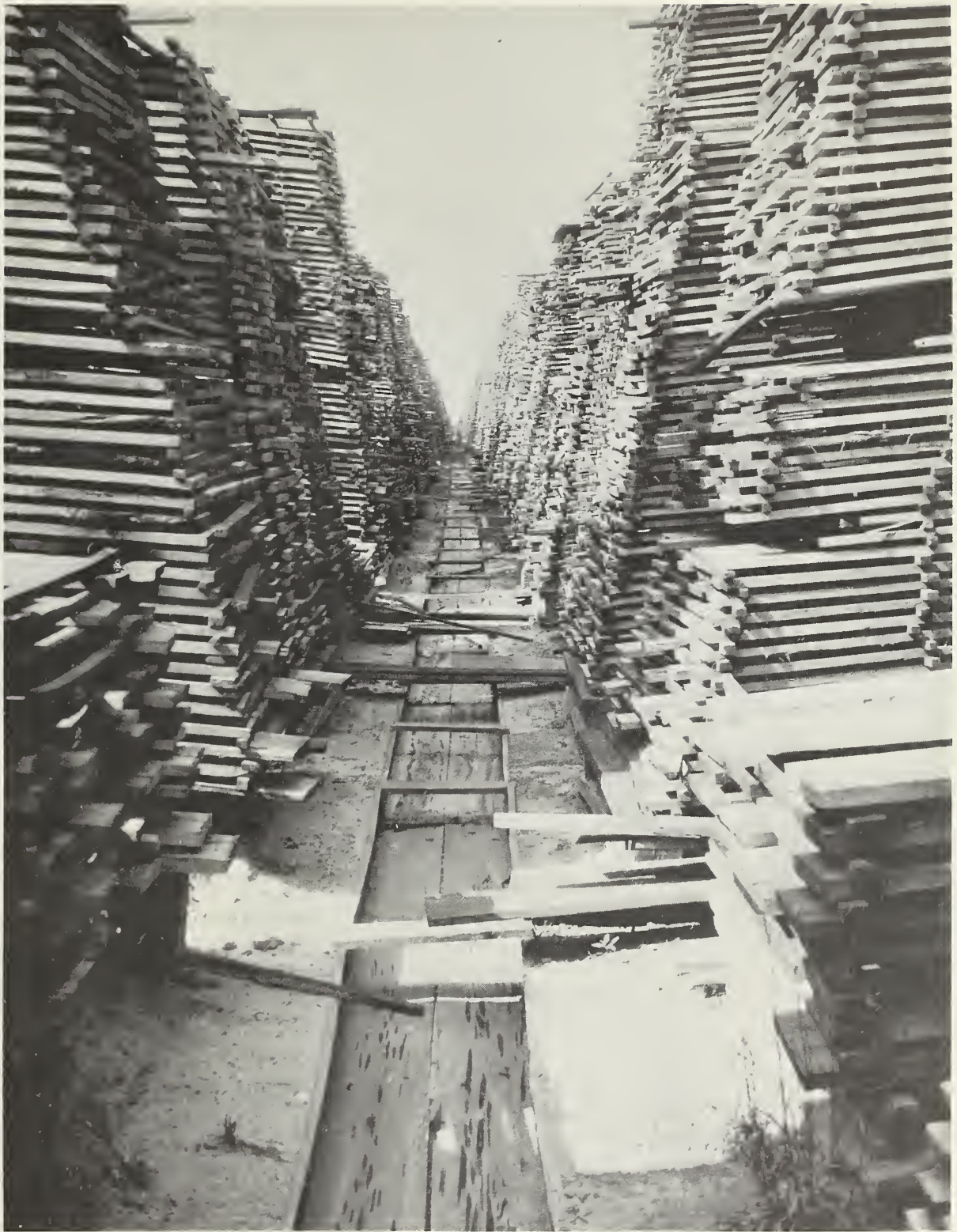
Figure 20. --Rear alley of a yard of handstacked piles, showing good drainage trough and generally good sanitation.
